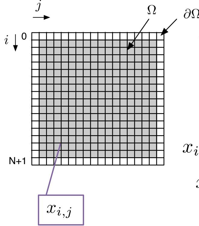
$$\begin{aligned}\nabla^2 \phi &= 0 \quad \text{on } \Omega \\ \phi &= f \quad \text{on } \partial\Omega\end{aligned}$$
