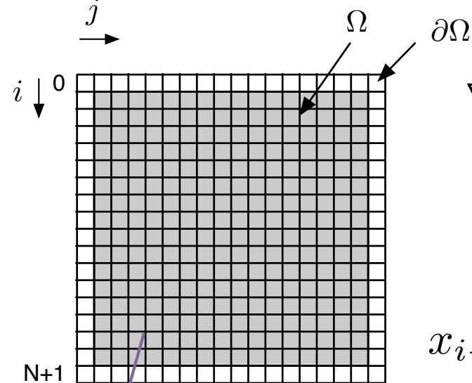
$$\begin{aligned}\nabla^2 \phi &= 0 \quad \text{on } \Omega \\ \phi &= f \quad \text{on } \partial\Omega\end{aligned}$$
